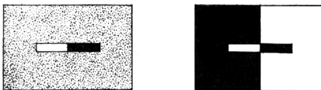
Fig. 4 White and black strips for simultaneous observation of regular and complementary spectrum
